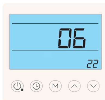
Fig.4 controller interface-Running parameter query
