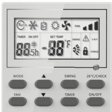
Fig1 Appearance of Wire Controller
